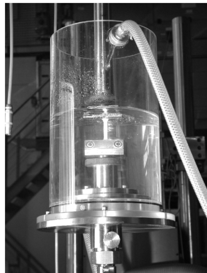
Fig. 8. Environmental chamber attached to servohydraulic testing machine.
